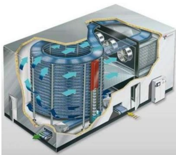
Figure 2 – Spiral quick freezer for freezing semi-finished dough products
